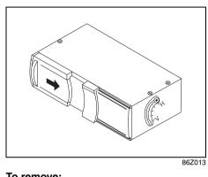
1) Open the sliding door of the CD changer to the right until it is completely latched.
